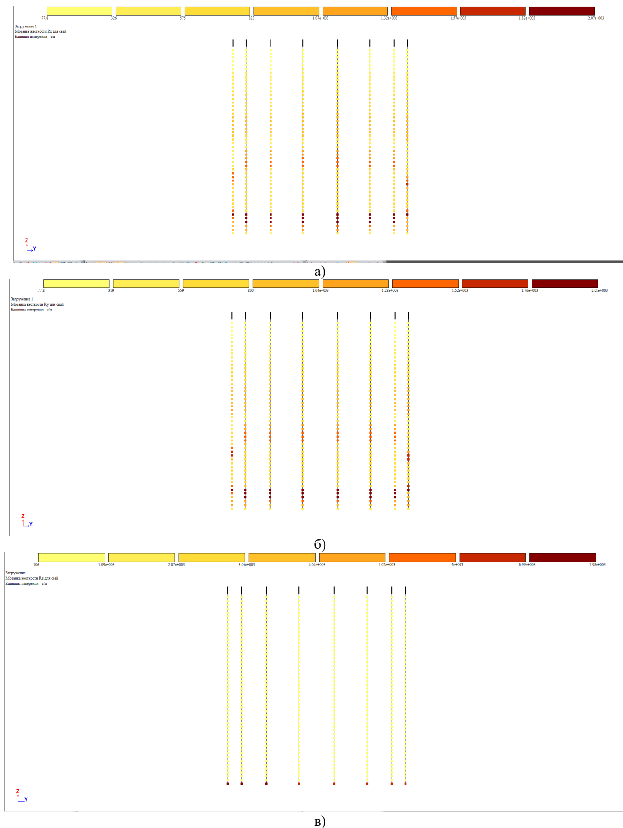
Fig. 4. Forces in piles: a – arising in piles along the X axis; b – arising in piles along the Y axis; c – arising at the ends of piles
