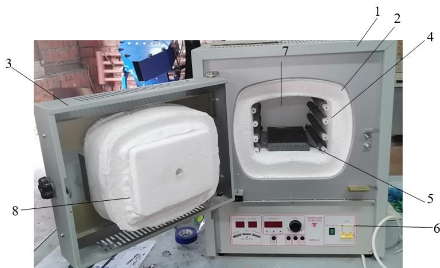
Fig. 1. Design of the muffle furnace: 1 – body; 2 – furnace muffle; 3 – door; 4 – heating elements; 5 – support plate; 6 – front control panel; 7 – thermocouple; 8 – door muffle.
