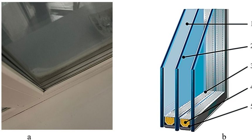
Fig. 4. Translucent window aperture: a – view of a in-place window; b – name of the translucent window aperture construction: 1-air chamber, 2-glass sheet, 3-distance frame, 4-molecular sieve, 5-sealant.
