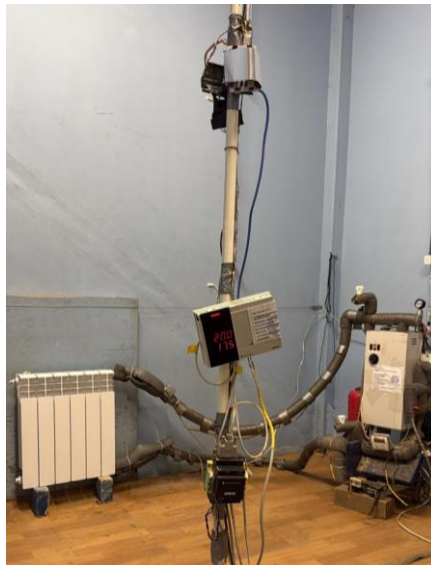
Fig. 3. Isothermal chamber with a laboratory stand for determining the nature of the temperature distribution in the study area, in the presence of spatial heat exchange.
