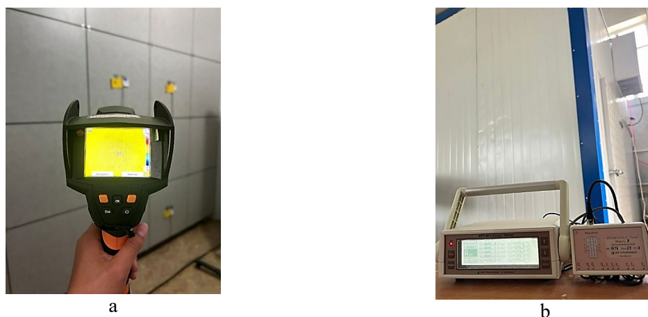
Fig. 6. Measuring instruments used in the experiments: (a) Testo thermal imager with analysis software; (b) ITP MG-4.03 heat flux density meter.
