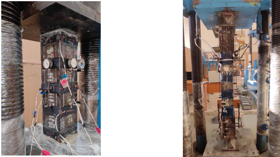
Fig. 5. Test setup configuration for 2500 kN and 5000 kN presses.
