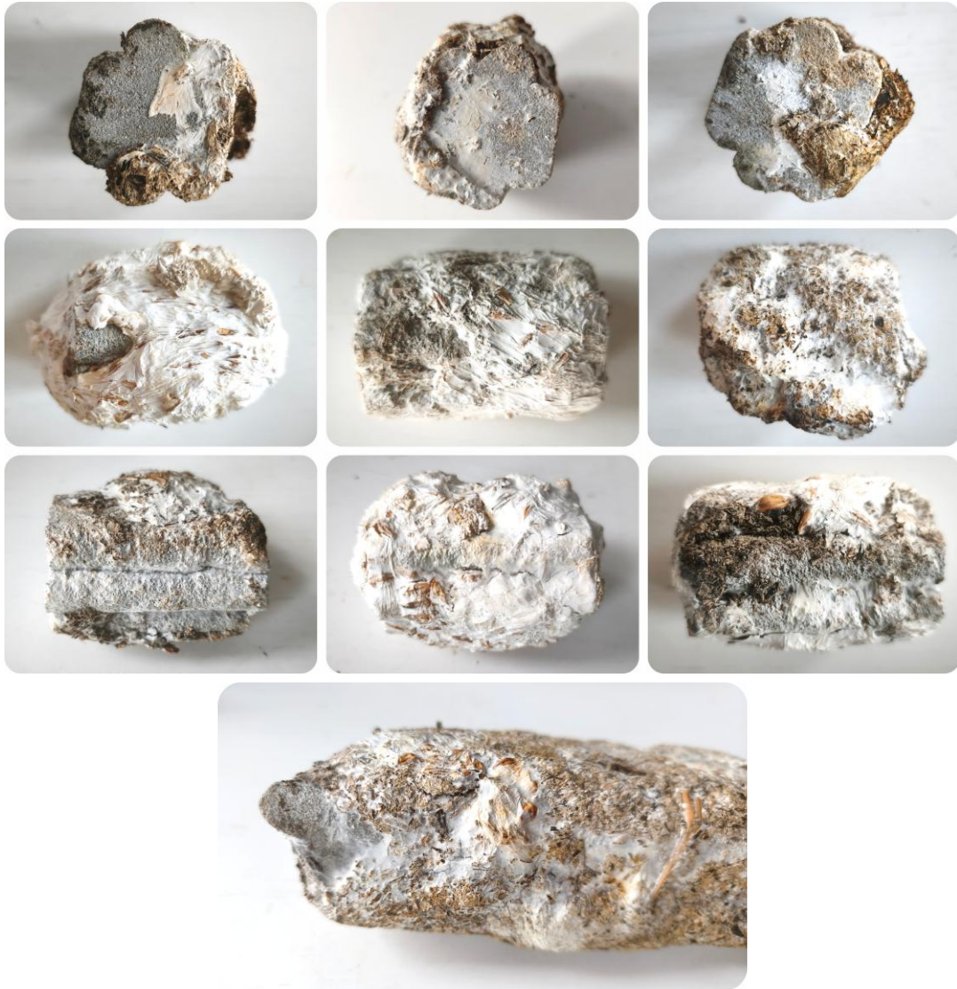
Fig. 10. 3D printed concrete structures elements, healed and reinforced with Mycokarst material. Author's image.
