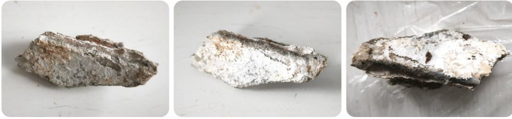
Fig. 9. Elements of a historical mineral brick facade healed and reinforced with Mycokarst material. Author's image.
