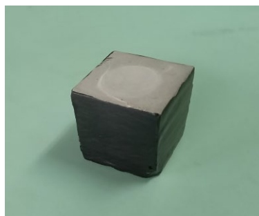
Fig. 1. Photo of a cement stone sample for corrosion testing.
