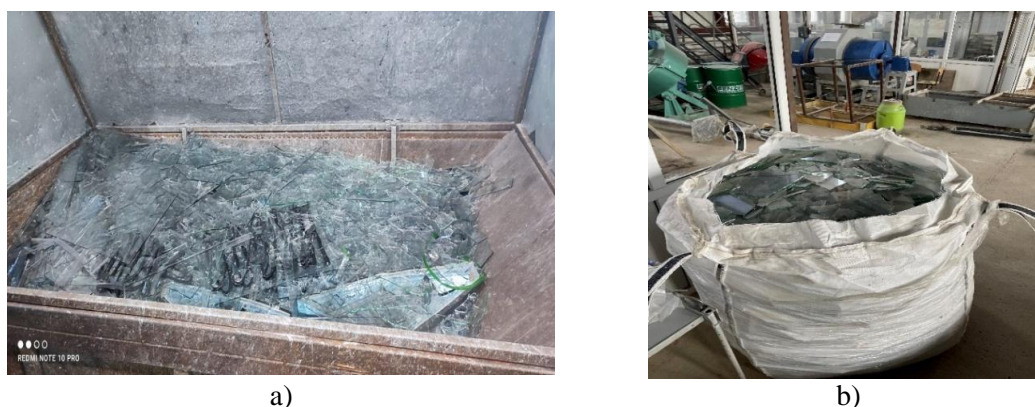
Fig. 1. General view of glass cullet generated by "Stekloservis," JSC: a – collected in metal containers, b – collected in big bags.
