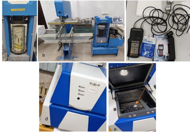
Fig. 5. a) Specimen, b) Testing machine C040PN, c) Ultrasonic device PULSAR-2.1, d) Clever C-31 (also known as RENOM FV), a universal X-ray fluorescence (XRF) spectrometer, e) Specimen.
