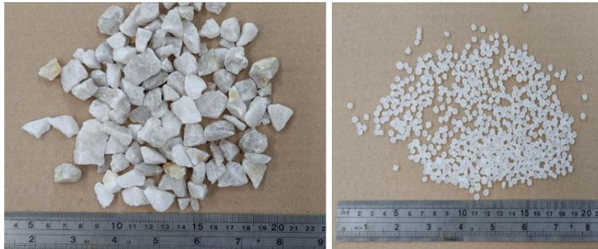
a) Vein quartz with a maximum nominal size of 20 mm. b) The granules of a specific size range (4-5 mm) of LDPE.
