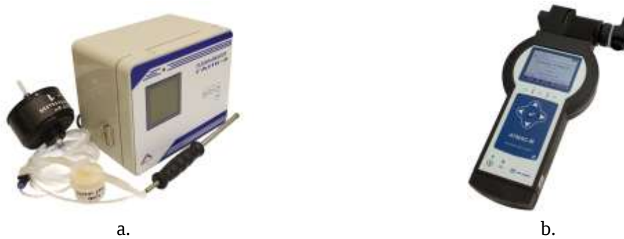
Fig. 2. Equipment used in the study: a – GANK-4 gas analyzer by NPO PRIBOR (Russia); b – portable analyzer, Atmos by ATMOS MedizinTechnik (Germany).
