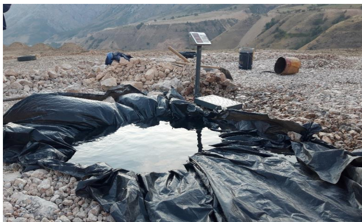
Fig. 2. Determination of the in-situ dry density of the first compacted layer using the pit-hole method after initial vibratory compaction.
