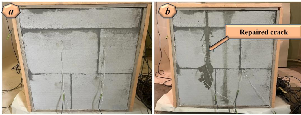
Fig. 3. Foam concrete specimens tested in the experimental apparatus: (a) intact specimen; (b) specimen containing a repaired crack.
