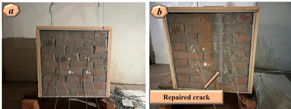
Fig. 5. Photographs of the specimens mounted in the developed test apparatus: (a) intact clay brick wall specimen; (b) clay brick wall specimen with an injection-repaired crack.
