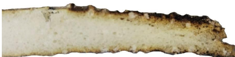
Fig. 11. Photograph of a cross-section of the composite sample after fire tests, composition with 90% SC, 0.9-1.25 mm fraction.
